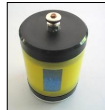
Non-polarizable electrode Cu – CuSO 4 500 g – 13 cm – 8 cm diameter
