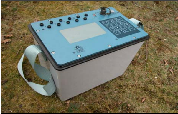
Elrec Pro Switch-48 unit with its graphic LCD screen
