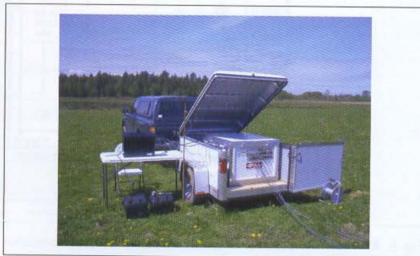
Fig 7. GeoMRI, 4-channel MRS instrument (April 2006)
