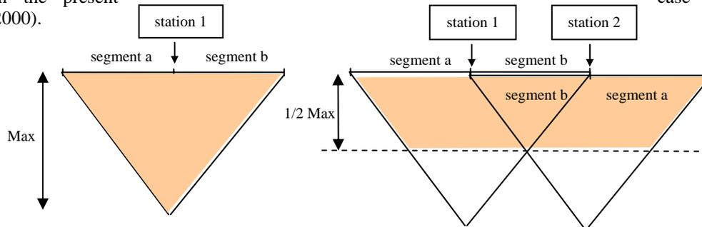
**Figure 3: Depth of penetration in multi-electrode resistivity measurements: simple configuration (on left); roll along configuration (on right)**
