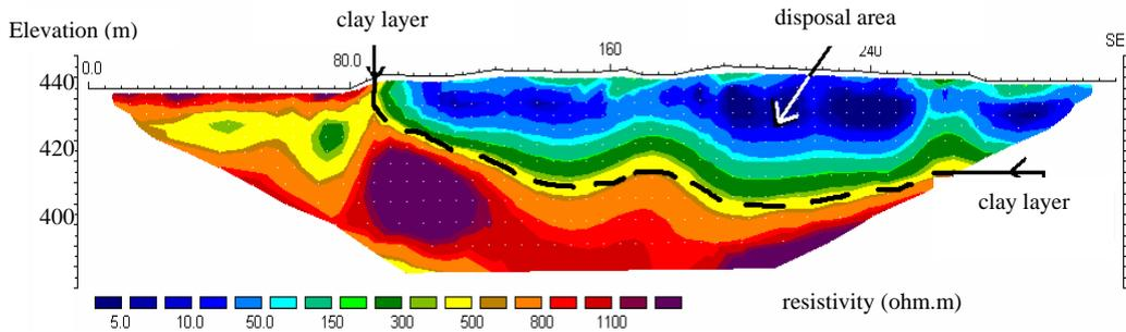
**Figure 7: Waste disposal area resistivity imaging (France)**
