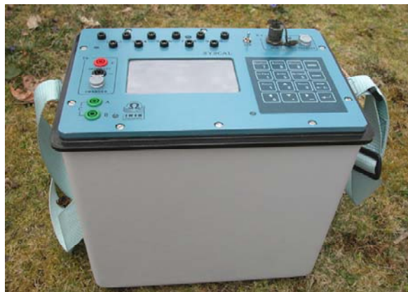
Figure 4 : SYSCAL Pro Switch, ten simultaneous channel multi-electrode resistivity system, with 250W , 800V and 2.5A outputs
