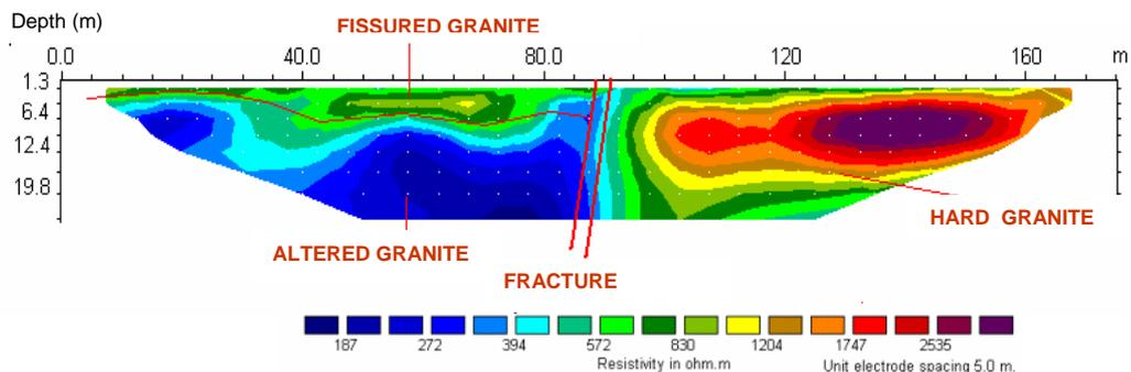
Figure 6: Fault resistivity imaging (Spain)
