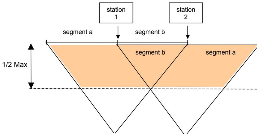
In case of a roll along procedure with a two segment cable (a and b), a first sequence of readings is taken with the equipment located in station 1, using the segments a and b.
