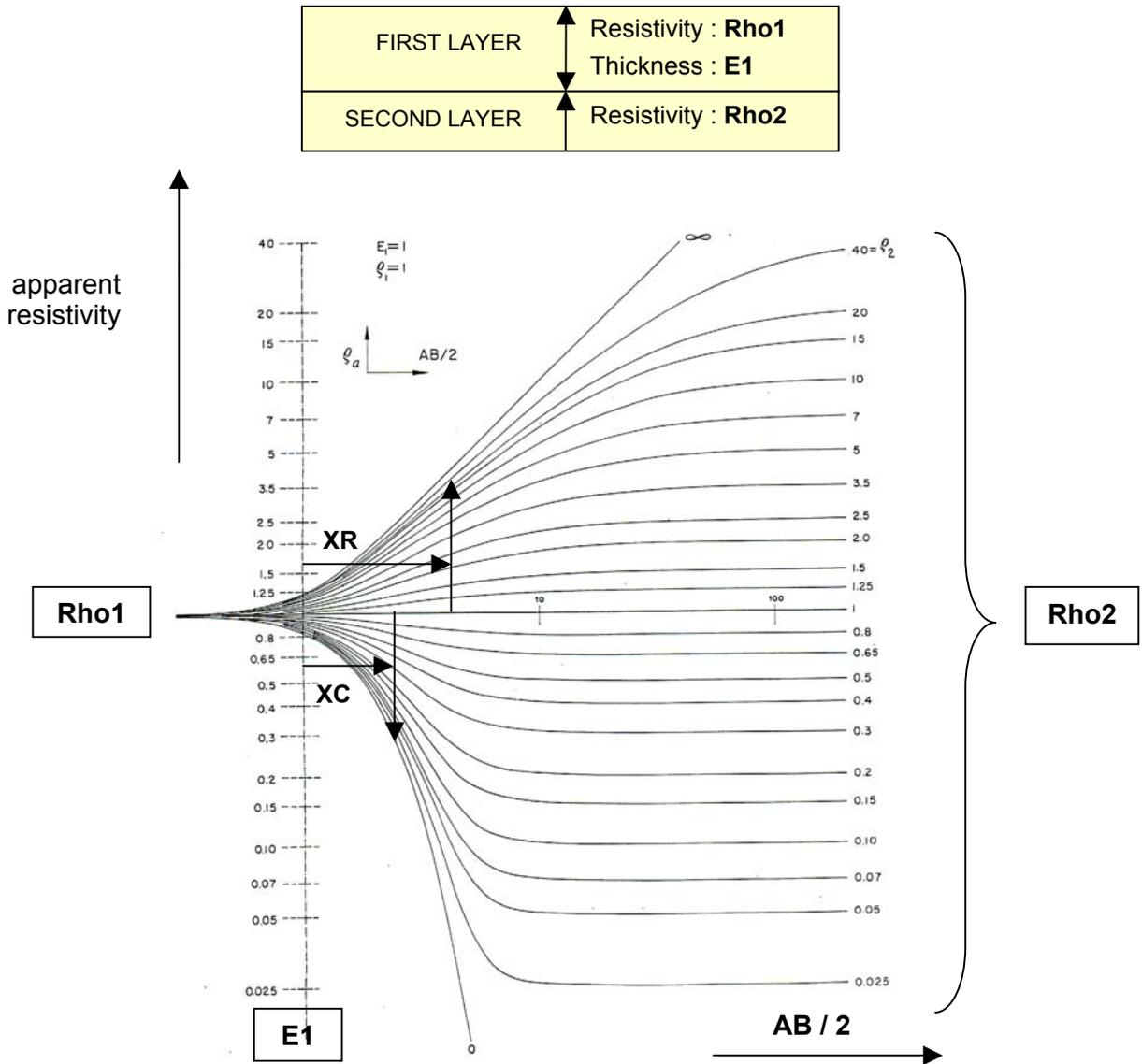
In case of a two layer sounding, when the second layer is more resistive than the first one, its presence is observed in the apparent resistivity curve for a length of line AB/2 longer than when the second layer is more conductive. In the figure, XR is longer than XC, for the same relative variation of the apparent resistivity curve.
