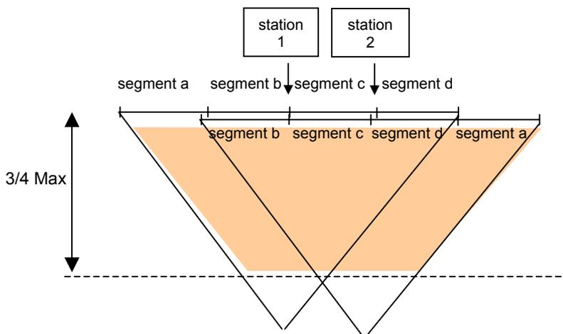
In case of a roll along procedure with a four segment cable (a, b, c and d), a first sequence of readings is taken with the equipment located in station 1, in the middle of the segments a, b, c and d.
