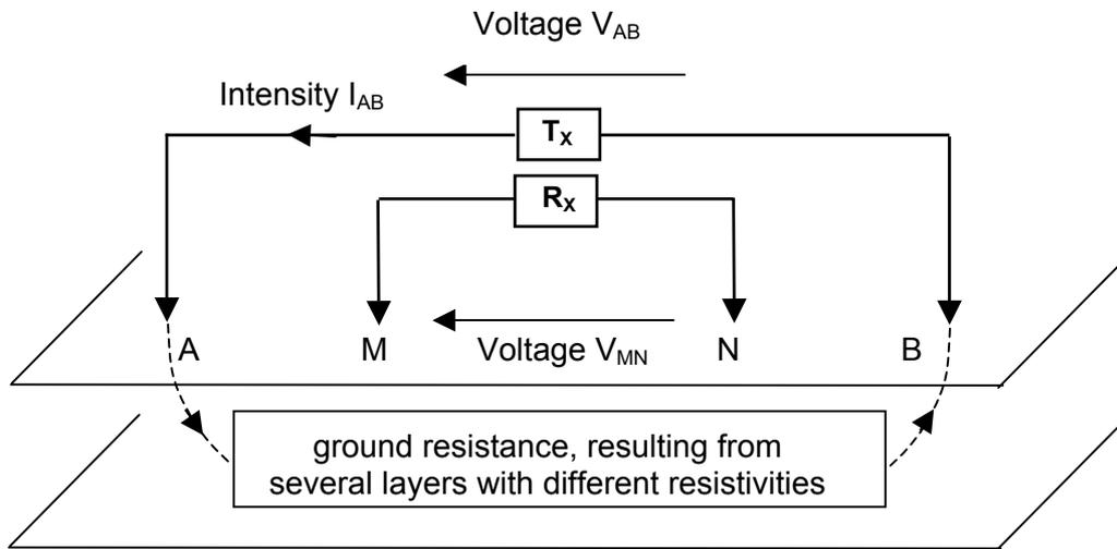
**APPARENT RESISTIVITY = (coefficient) x voltage / intensity =  $\rho = K \times V_{MN} / I_{AB}$**
