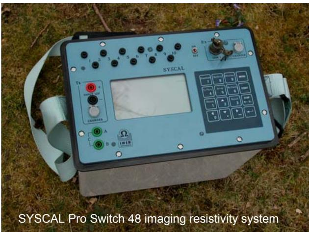
SYSCAL Pro Switch 48 imaging resistivity system
