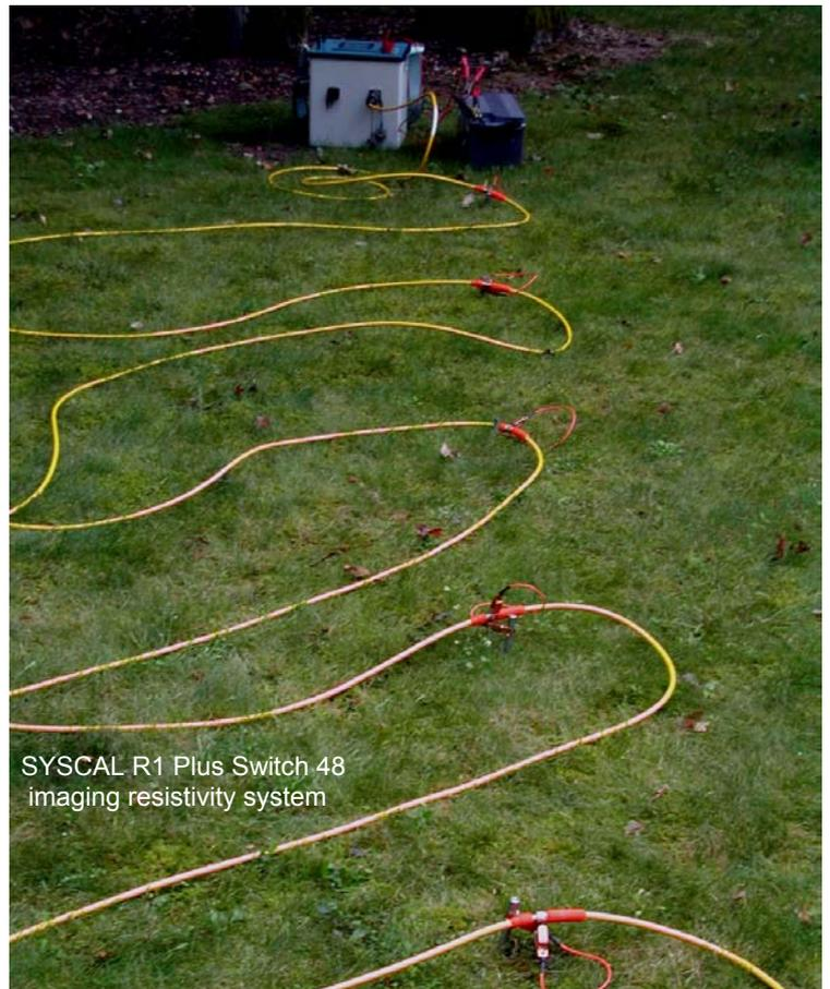
SYSCAL R1 Plus Switch 48 imaging resistivity system
