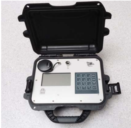
V-Full Waver , compact recorder for full wave signal
