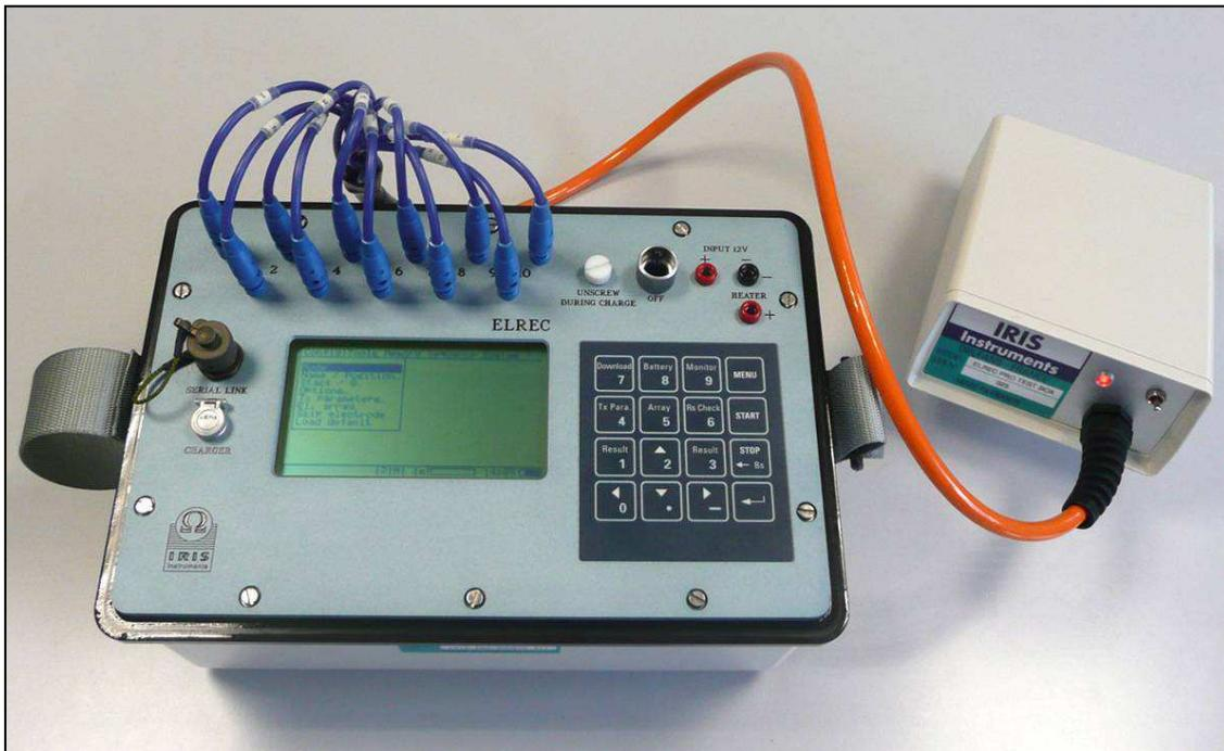
This test box is not a calibration unit, but a test unit which aims at checking the good operation of an ELREC Pro receiver. It allows to control the **Rs Check function** and the **measuring function** of an ELREC Pro for each channel.
