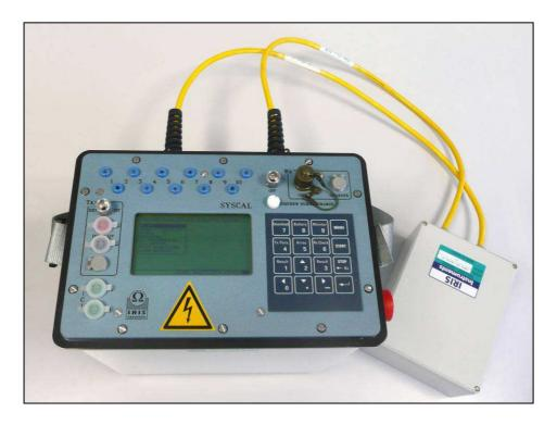
This test box is not a calibration unit, but a test unit which aims at checking the good operation of a SYSCAL Switch or a SYSCAL PRO Switch version. It allows to control the **Rs Check function** and the **measuring function** of a SYSCAL for each channel.
